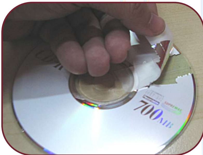
Fig. 10: Removing the metal layer of the CD with adhesive tape.
