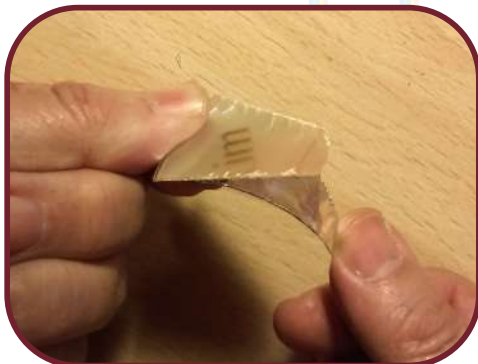
Fig. 16: Folding the piece of DVD separates the silver part of the used grid.
