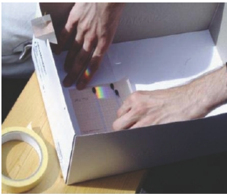
Fig.4: Placing the 3 thermometers, with the black bulb and the spectrum in the shadow.
