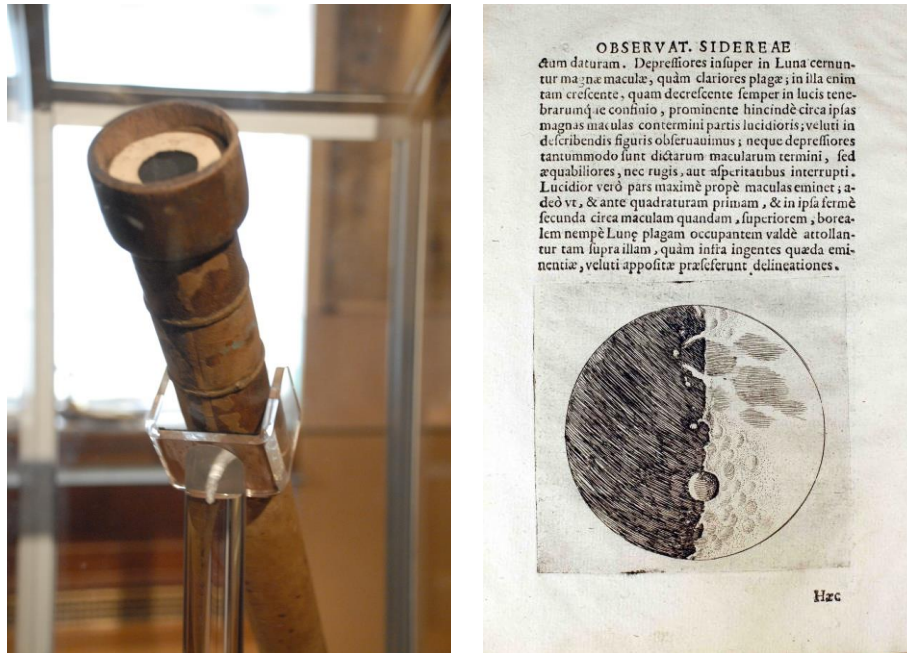
Fig. 7a: One of Galileo's two surviving telescopes came to the Franklin Institute in Philadelphia in 2009, on its first visit to the United States. Note that the outer part of the lens is covered with a cardboard ring. By hiding the outer part of the lens, which was the least accurate part, Galileo improved the quality of his images. (Photo: Jay M. Pasachoff). Fig. 7b: A page from Galileo's Sidereus Nuncius (The Starry Messenger), published in 1610, showing an engraving of the Moon. The book was written in Latin, the language of European scholars. It included extensive coverage of the relative motion of the four major moons of Jupiter.
