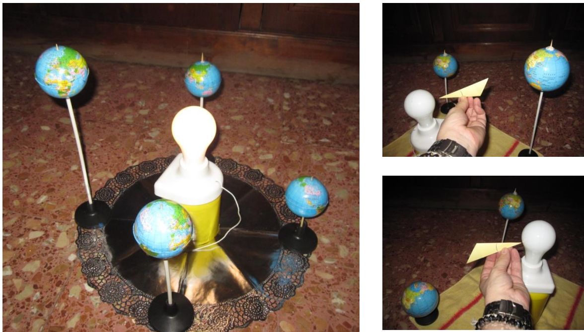
Fig. 2a, 2b and 2c: Distribution of the four spheres representing Earth and the light bulb representing the Sun, in the middle. It is necessary to distribute the relative positions so that the angle of the line from the center of the Sun to the center of the Earth is 23^\circ with respect the ground that represents the equatorial plane.
