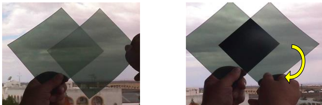
Fig. 4a: If the filters have the same orientation, light passes through, Fig. 4b: If one of the filters is turned 90°, light is blocked.
