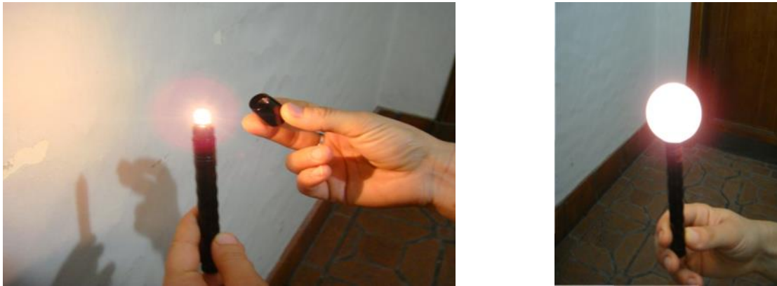
Fig. 15a: We removed the protector of the flashlight, Fig. 15b: Flashlight with the tennis table ball simulating the street lamp
