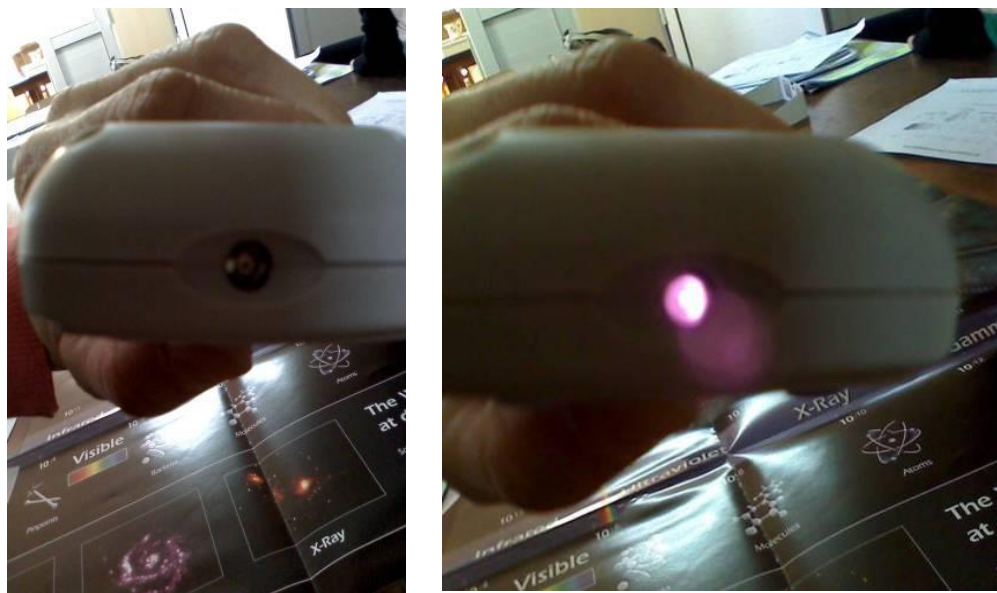
Fig. 10a: Remote activated naked eye, Fig. 10b Remote activated by mobile phone.
