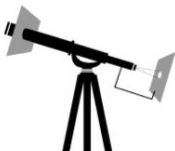
Fig. 10a: Solar observation by projection with a telescope (never look directly at the Sun), Fig. 10b: Observation by projection with binoculars (never look directly at the Sun).
