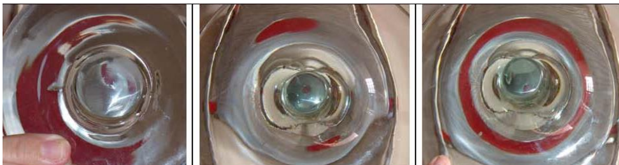
Fig. 24a, Fig. 24b and Fig. 24c: The glass foot can simulate various shapes made by gravitational lenses: arc segments, images of points, and Einstein rings.
