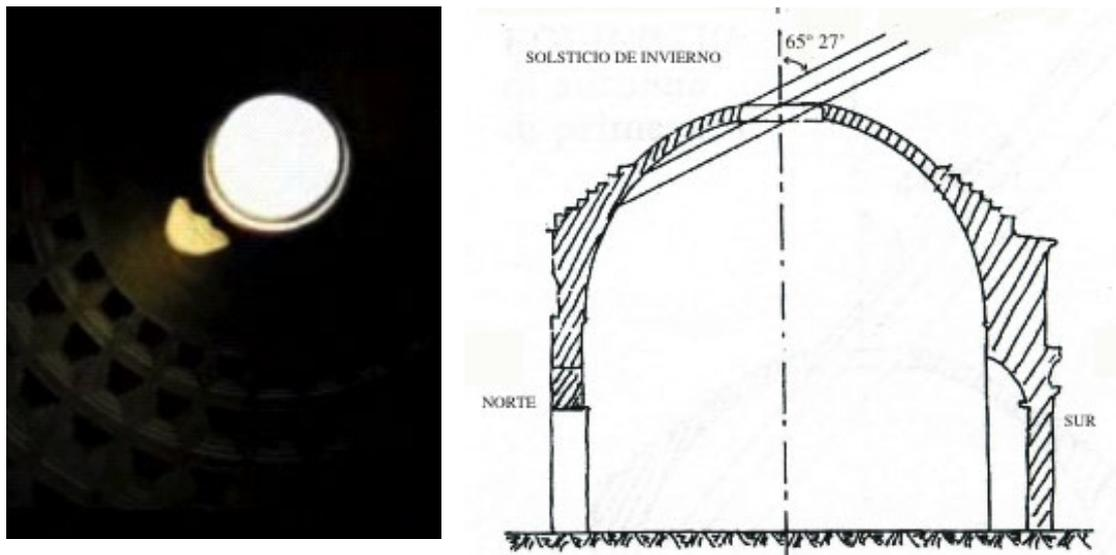
Figure 7: Winter Solstice. The light spot falls on the top of the dome.
