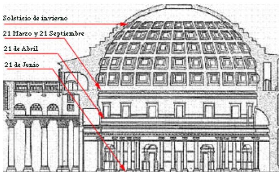
Figure 5: Elevation section of the Pantheon where it represents how impinging rays of the Sun at the solstices and equinoxes.
