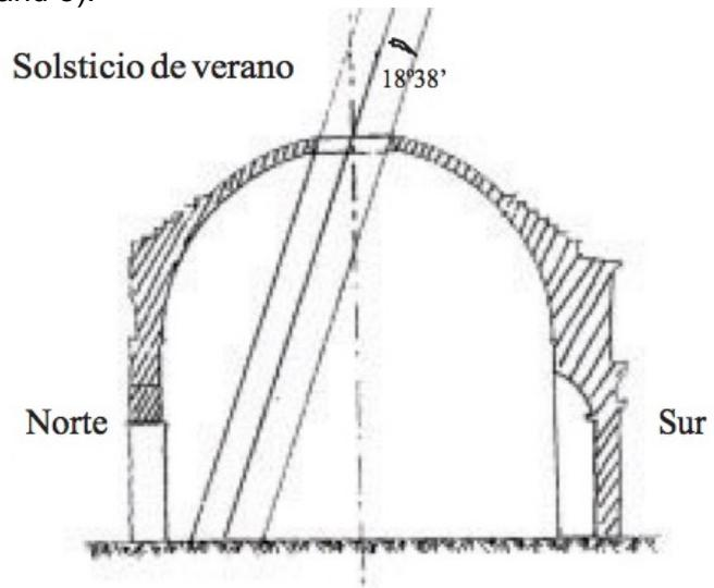
Figure 8: Summer Solstice. The light spot falls on the pavement of the dome.
