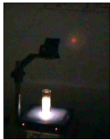
Fig. 24c: When the glass is full, the light reaching the wall is red
