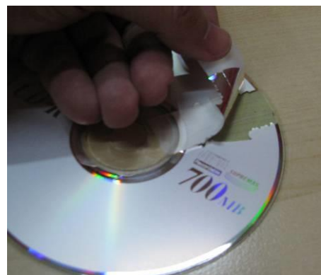
Fig. 3b: Removing the metal layer of the CD, with tape.
