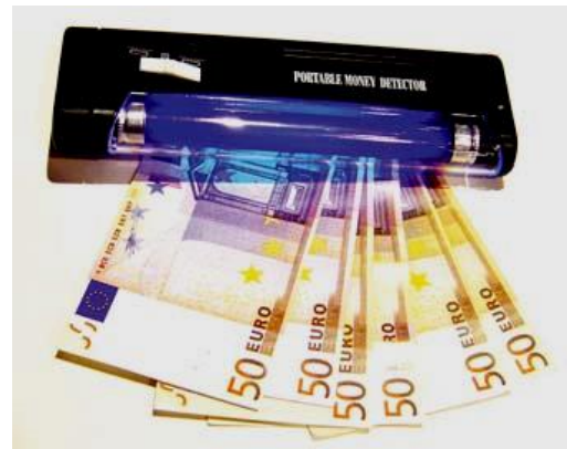
Fig. 18: Counterfeit Detector, which uses ultraviolet light
