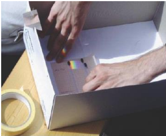
Fig.9a: Placing the three thermometers, with the black bulb, and the spectrum in the shadow part.
