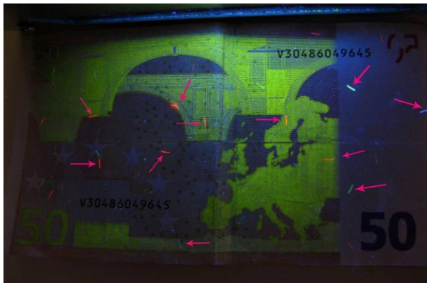
Fig. 17: A note of 50 € illuminated with UV light, shows small fluorescent strips marked here by arrows.
