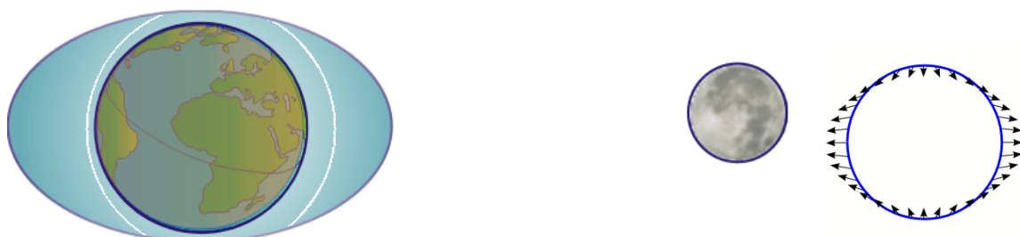
Fig. 20: Tide's effect. Fig. 21: Effect on water of the differential relative acceleration of the Earth in different areas of the ocean.
