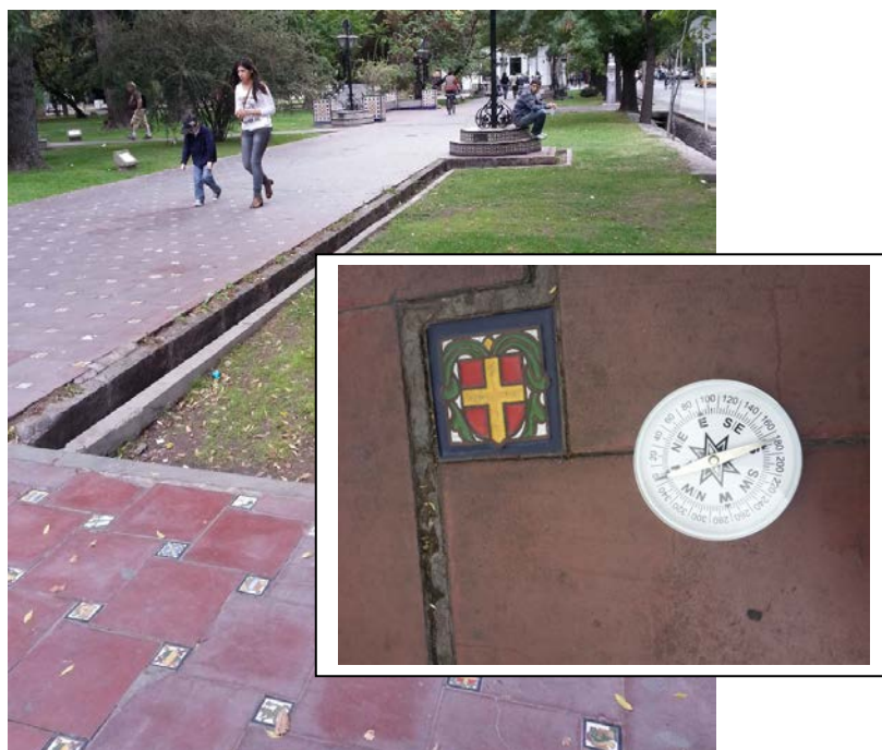
Fig. 25: Determination of the orientation of the North-South direction in the Plaza España. As you can see, the North-South direction forms an angle of about 20 degrees with the line of the tiles.
