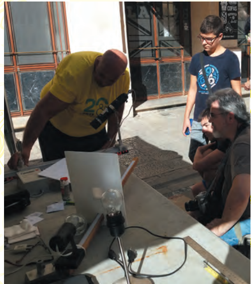
Using the Jacob's device adapted for measure the Power of the Sun. We can see the bulb at the end of the main stick and the white PVC perpendicular to it.
