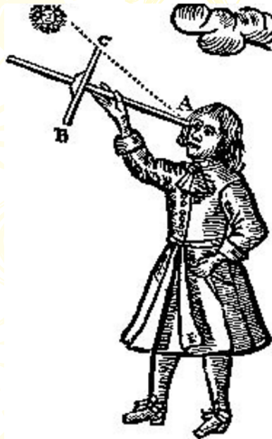
An ancient observer using a Jacob's staff
