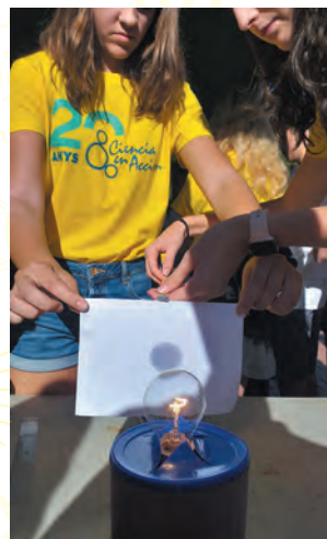
FBunsen photometer with the oil paper and detail of the oil stain
